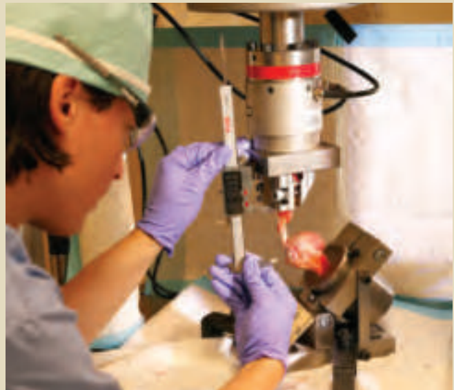
The biomechanical tests were performed in real-time using the Instron Electro-Puls E1000, allowing researchers to visibly see how well each surgical technique performed during testing procedures.
